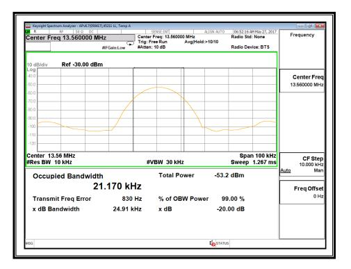
NOTE: Because the measured signal is CW adjusting the RBW per C63.10 would not be practical since measured bandwidth will always follow the RBW and the result will be approximately twice the RBW.
