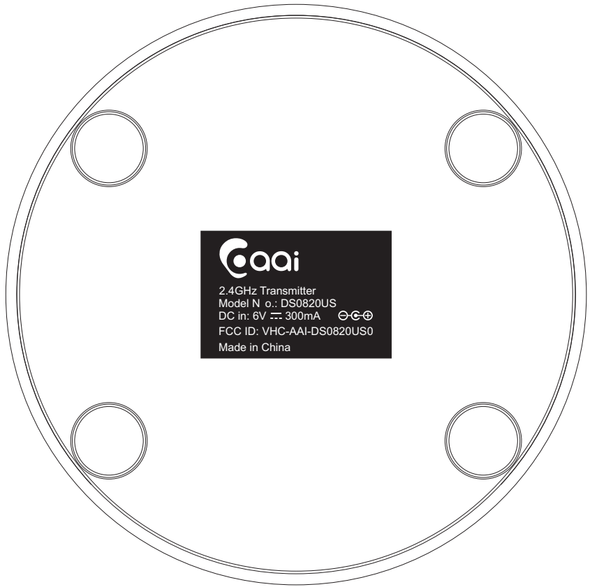
Transmitter rating label Size: 24x36mm Scale 1:1
