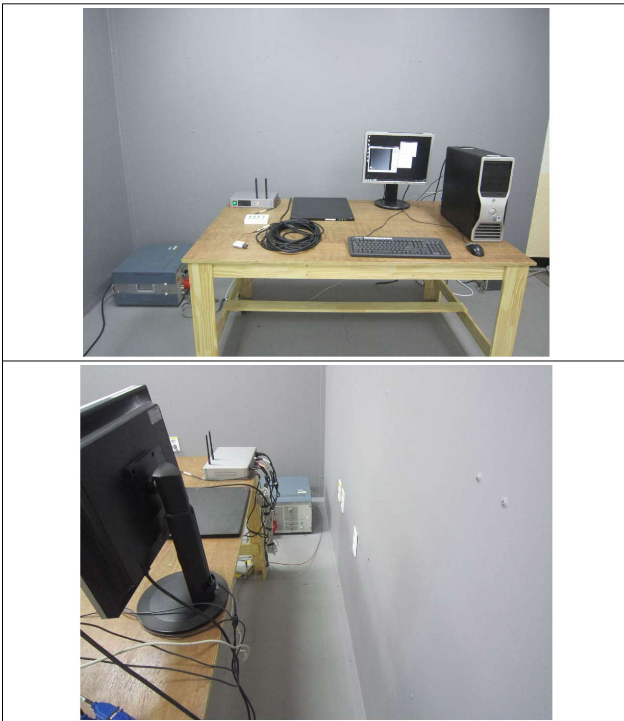
Figure.2. Test Setup for Conducted Emissions
