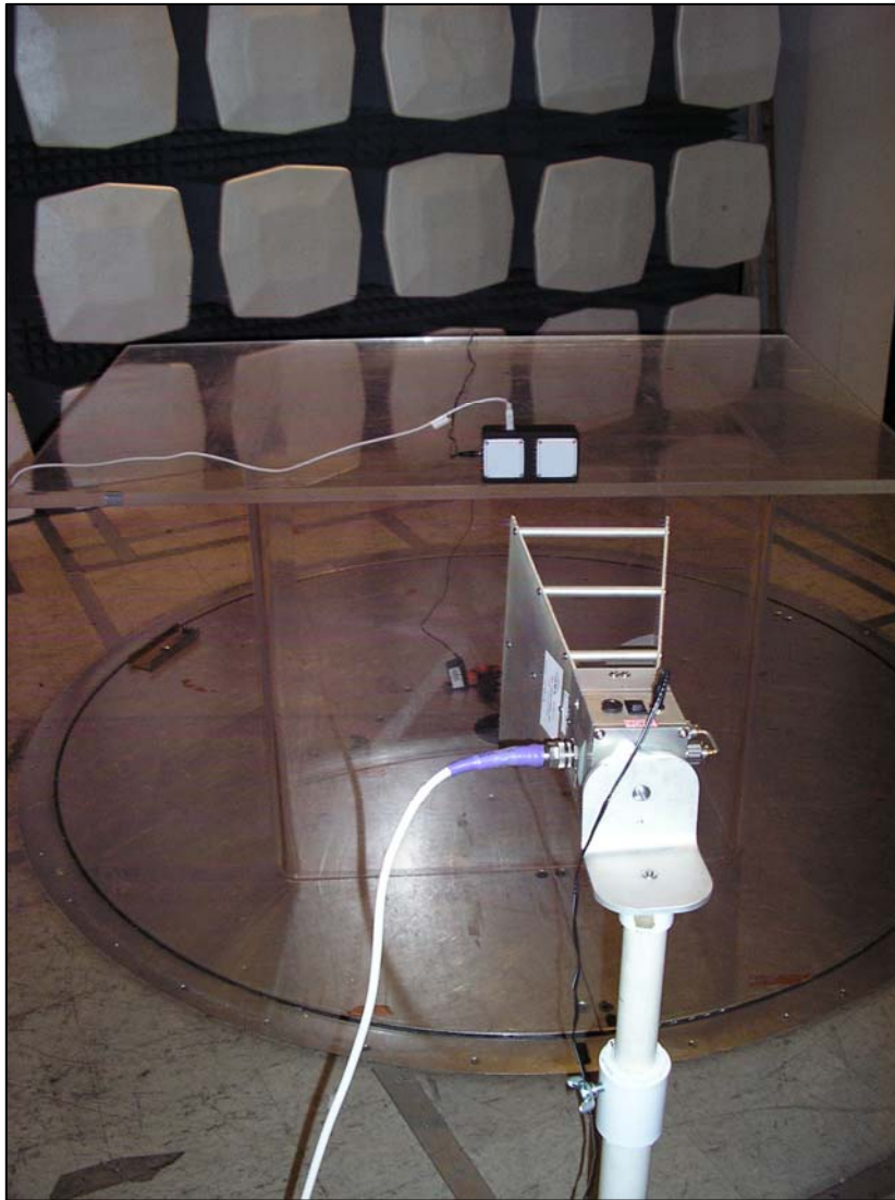
Photograph 6. Average Radiated Emissions Requirements – Narrowband, Test Setup
