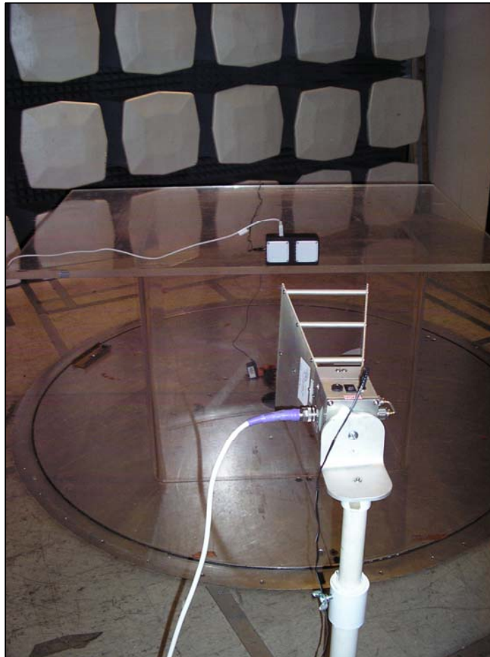
Photograph 4. -10 dB Bandwidth, Test Setup
