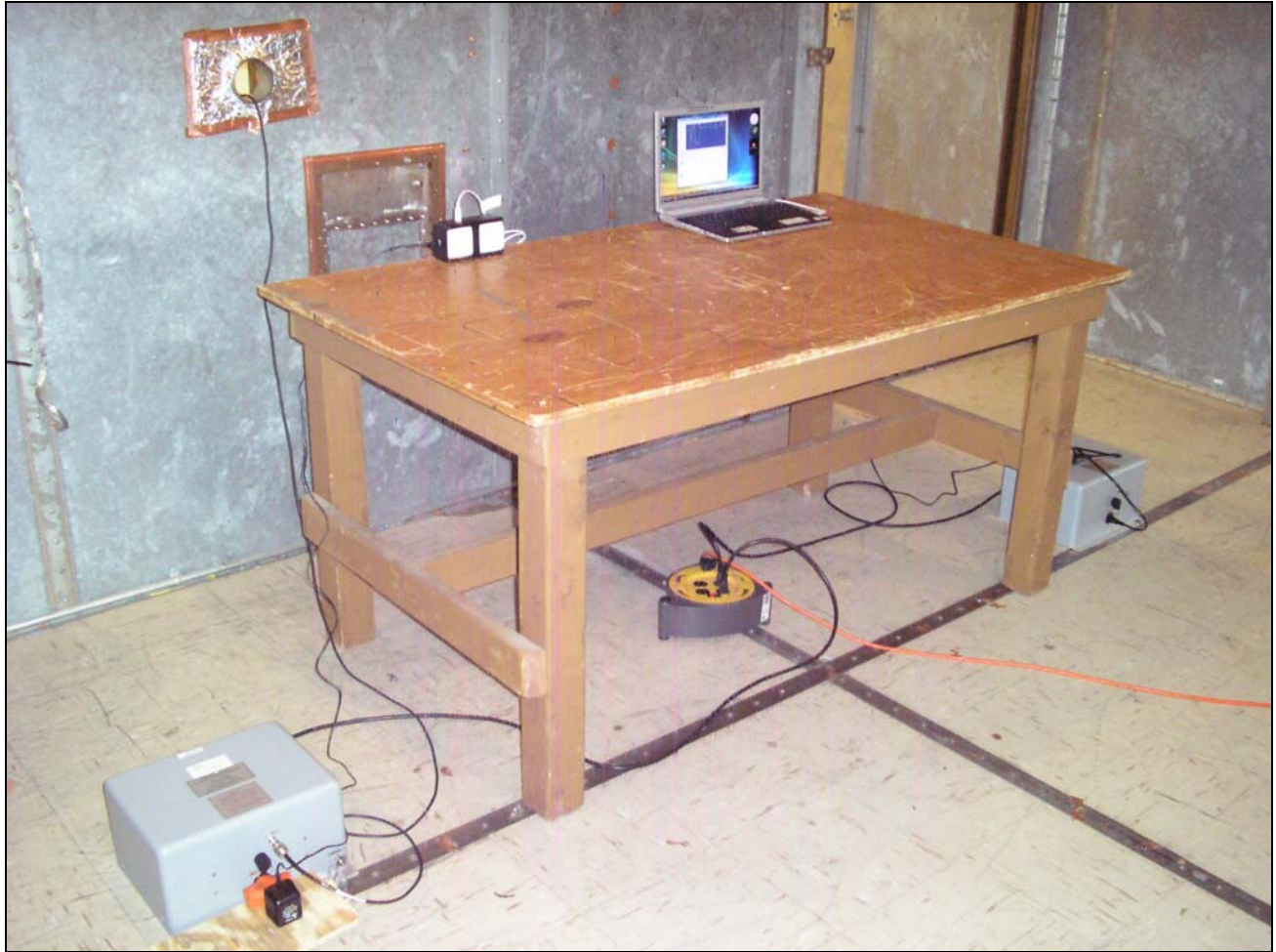
Photograph 3. Conducted Emissions, Test Setup
