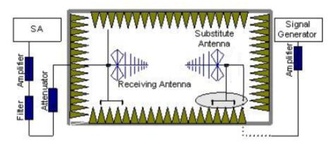
For 850MHz working frequency test
