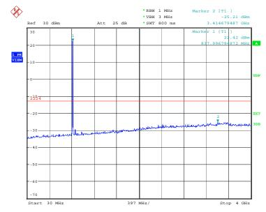
NOTE: peak above the limit line is the carrier frequency.
