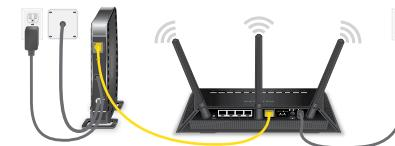
Unplug your modem, remove and replace the backup battery if it uses one, and then plug the modem back in. Use the Ethernet cable to connect the modem to the yellow Internet port on the router.
