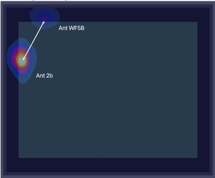
Figure 11-9 Back Side Spatial Separation for Antenna 2b and Antenna WF5B
