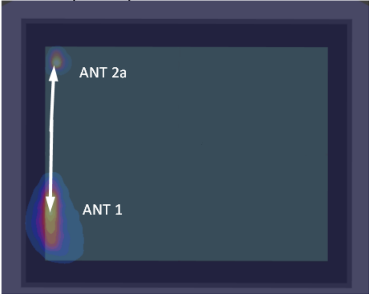
Figure 11-1 Back Side Spatial Separation for Antenna 1 and Antenna 2a
