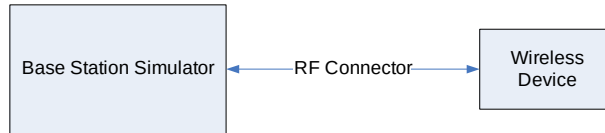
Figure 8-1 Power Measurement Setup
