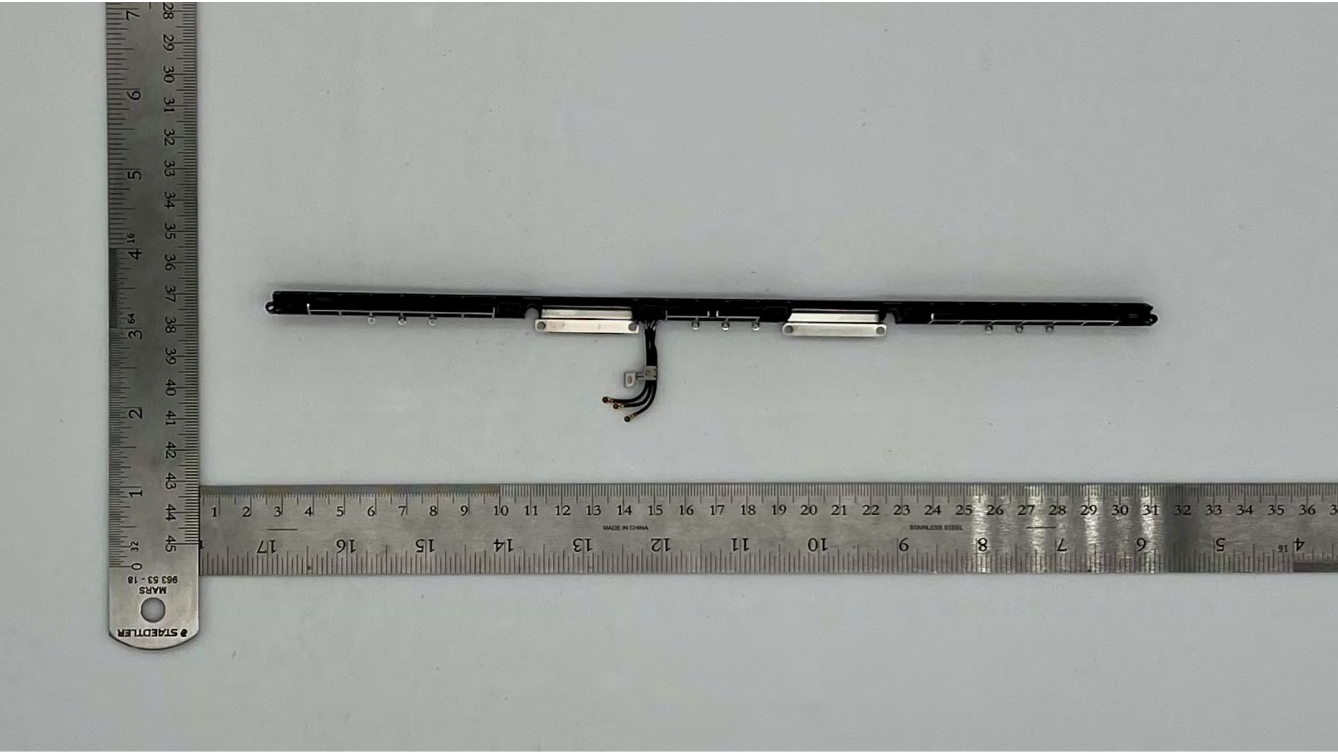
A2780 WF1/BT, WF2/BT, WF3 (BT) antenna structure and feed- Back
