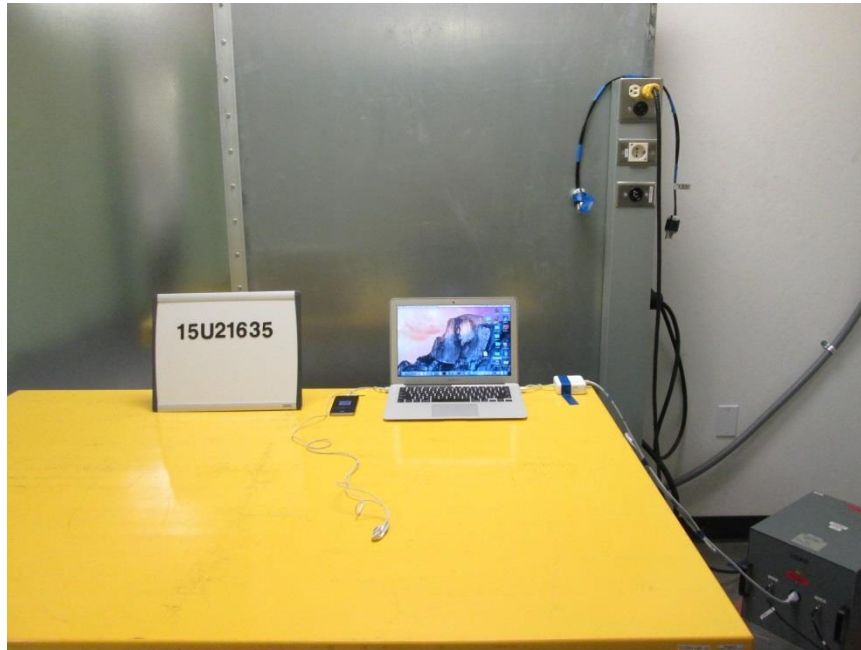
EUT WITH LAPTOP LINE CONDUCTED FRONT PHOTO
