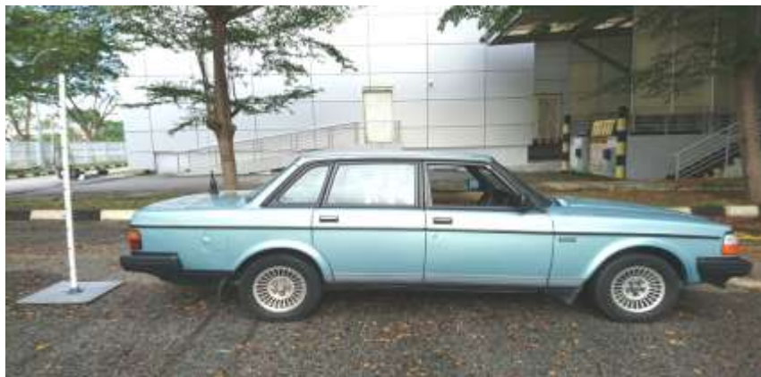
Test measurement setup for Bystander, trunk mount antenna behind vehicle
