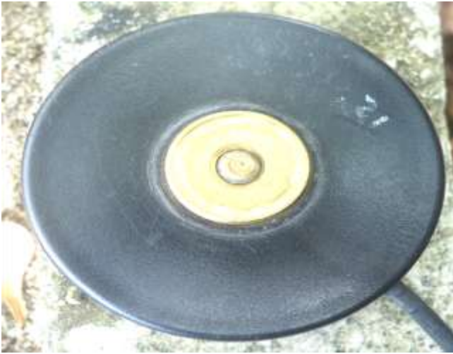
Magnetic mount base (top and side view)
