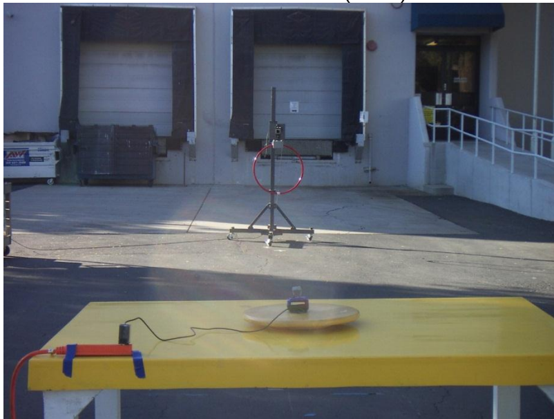
RADIATED EMISSIONS BELOW 30MHz (BACK)
