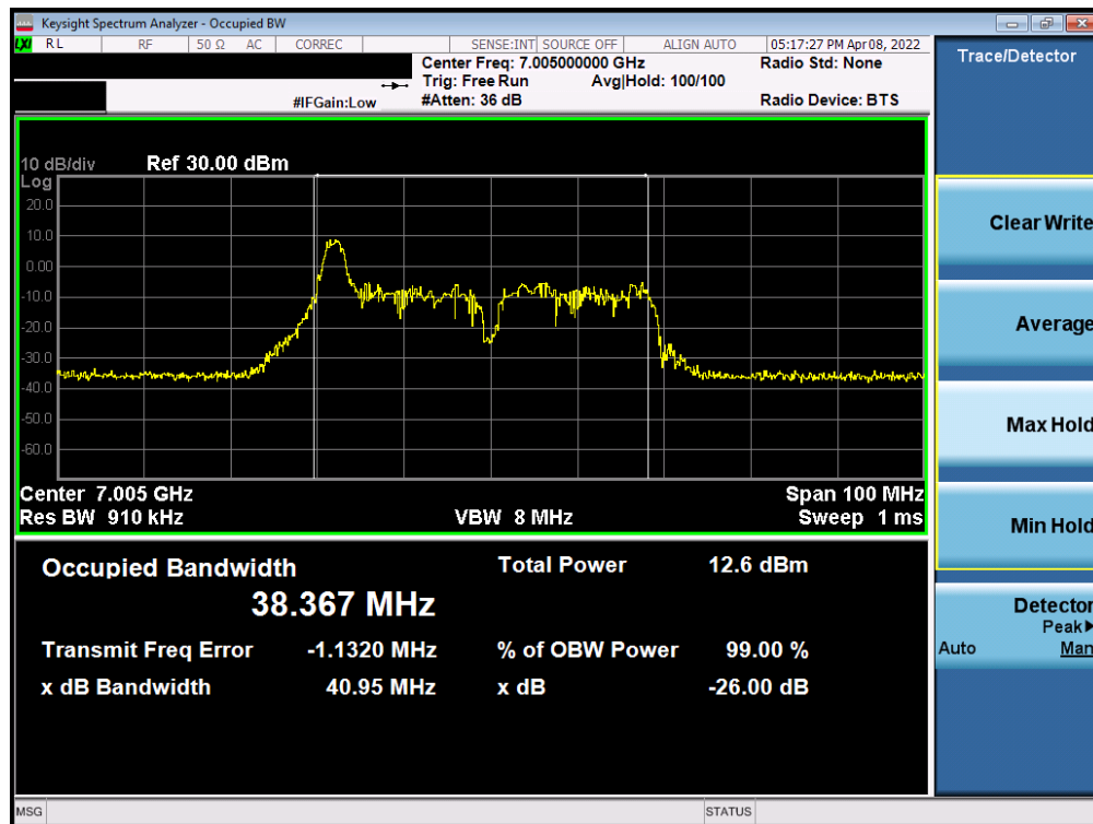
Plot 7-110. Occupied Bandwidth Plot MIMO ANT2 (40MHz BW 802.11ax (26 Tones) (UNII Band 8) – Ch. 211)
