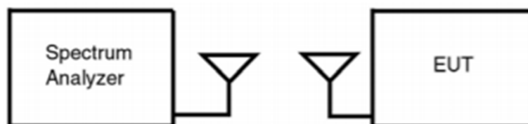
Figure 7-1. Test Instrument and Measurement Setup
