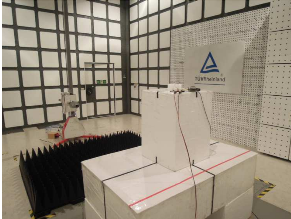
Photograph 13: Set-up for Spurious Emissions (Front View 1)- RFPCA381013IMAB701-ANT
