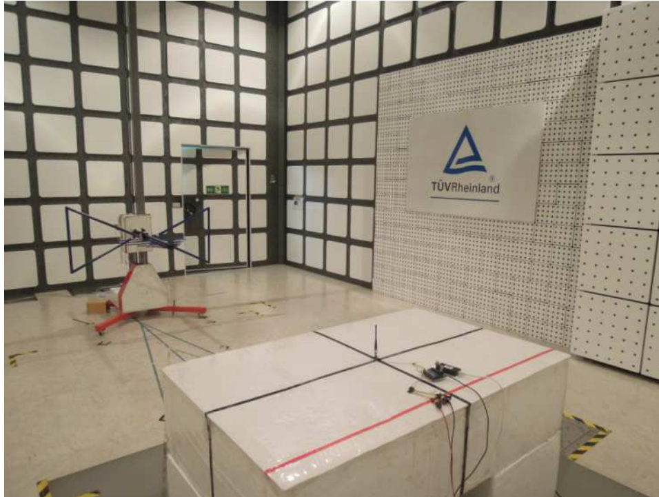
Photograph 3: Set-up for Spurious Emissions (Front View 2)- RFA-02-5-C7H1-ANT
