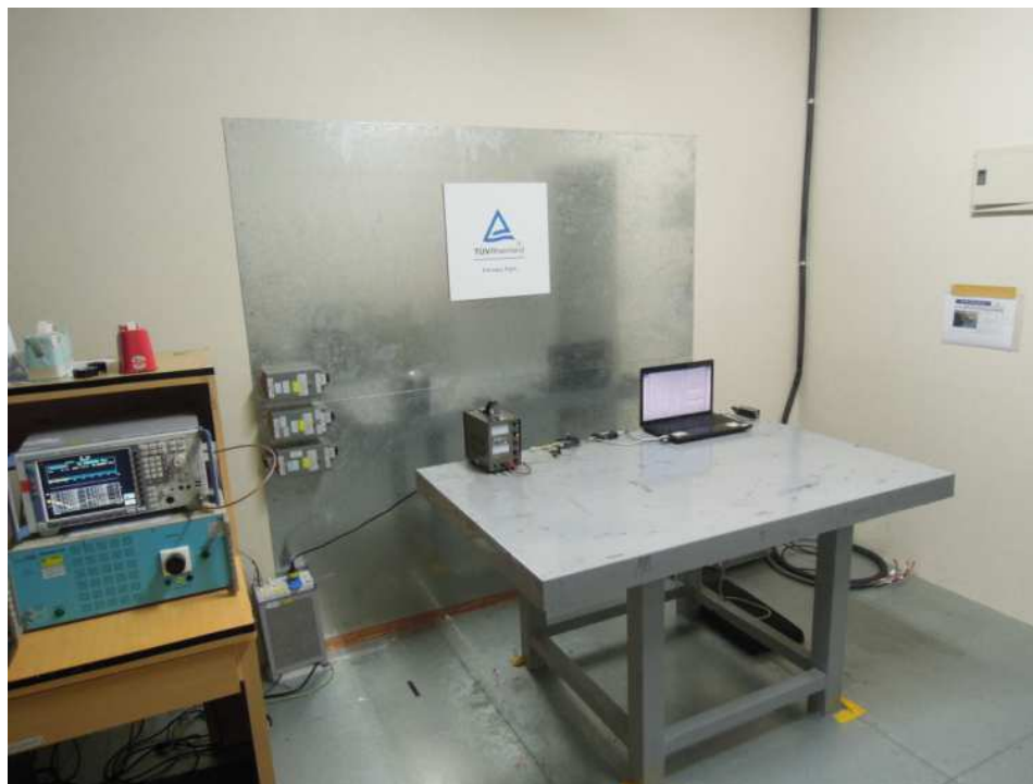
Photograph 21: Set-up for Mains Conducted testing (Front View)
