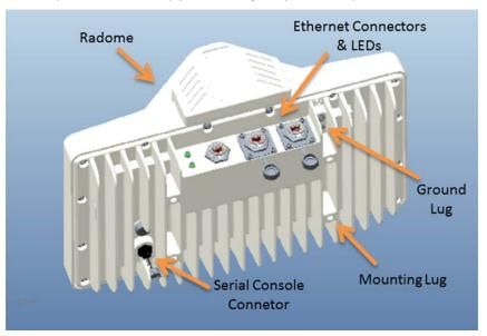
The side where the mounting lugs and serial port are located is referred to as the "back", since it is the side that will be against a wall or mast when IBR is mounted.
